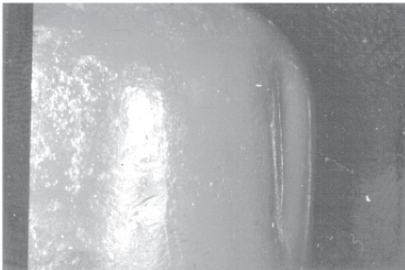
Figure C.1 — Cut or gouge
