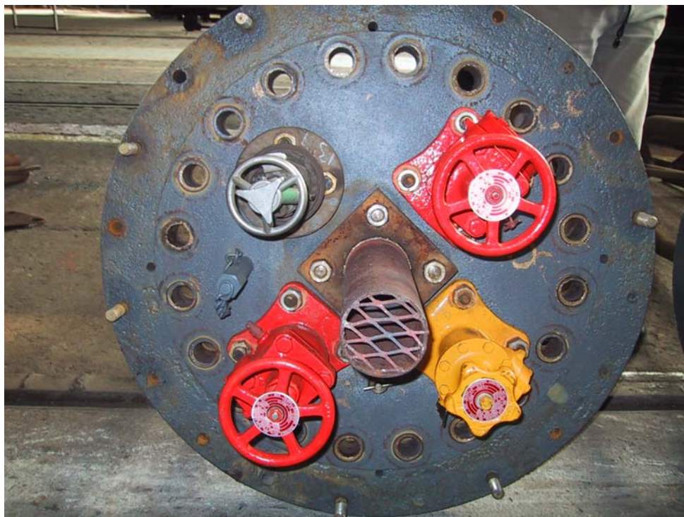
Figure 1 — Typical valve arrangement on rail tank cars
