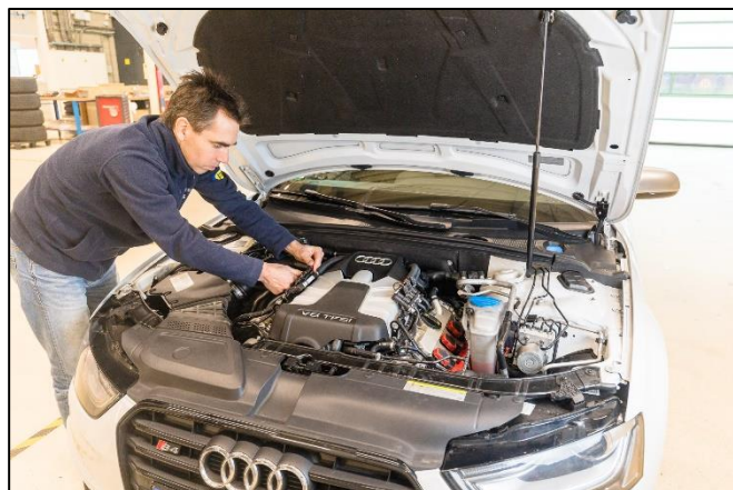
Installing an LPG system (courtesy - Prins)
